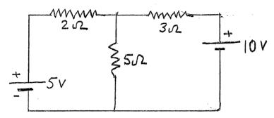
7-3. In the circuit shown,  $I_1 = 3amp$  and  $\varepsilon$  and R are not given. Calculate  $I_2$  and  $I_3$ .
