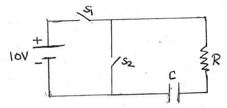
7-8. A long time later the switch  $S_1$  in the circuit of problem 7-7 is opened and  $S_2$  is closed, now calculate  $V_C$  and i at times (i) 0.1sec (ii) 0.3sec and (iii) 1sec after opening the switch. [Indicate direction of current].
