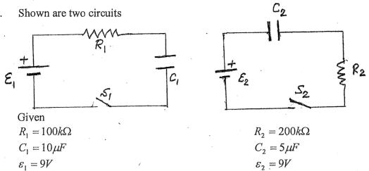
If both switches are closed at t = 0, which capacitor voltage will reach 6V first? Why?
